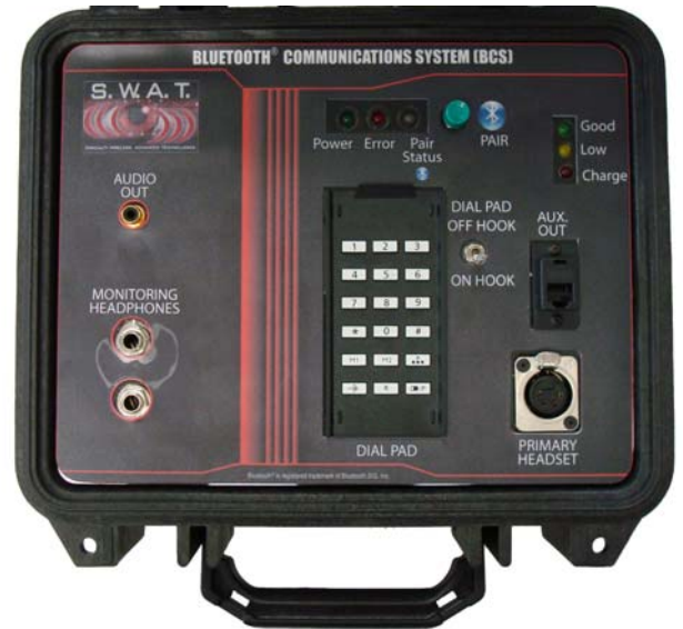
Bluetooth® Communications System (BCS) (Open/Top View)
